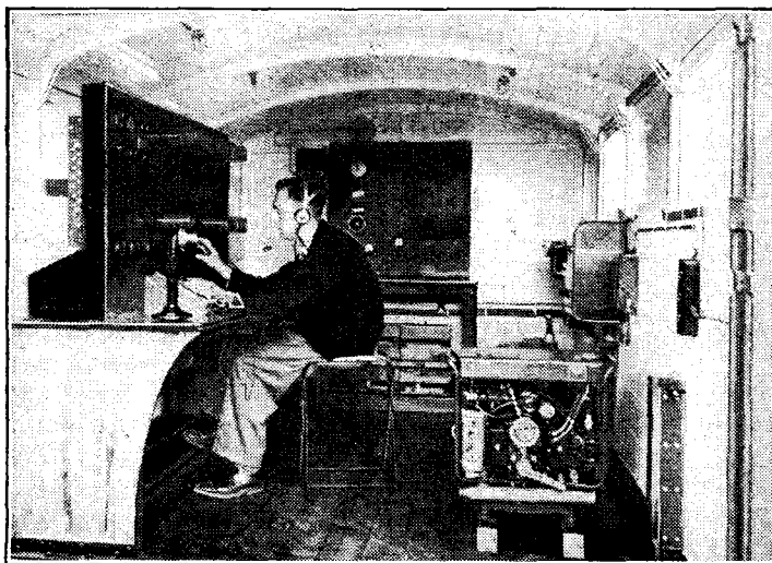
Mobile wireless station used by the Air Ministry for aircraft services at provincial aerodromes (Marconi).
